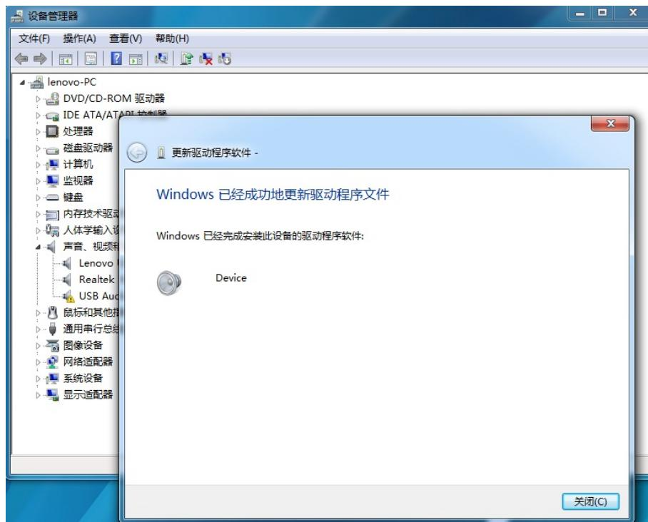
14: Go back to USB Audio Device under Device Manager and you will find now it's showing as a sign of Speaker and no name and ? mark is available. It means the driver is installed in your PC successfully. Thanks for your kind patience to read this driver installation instructions.
